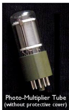
Photomultiplier tube with its protective covering removed. The sensitivity of the detector depends on the photocathode substance used.
