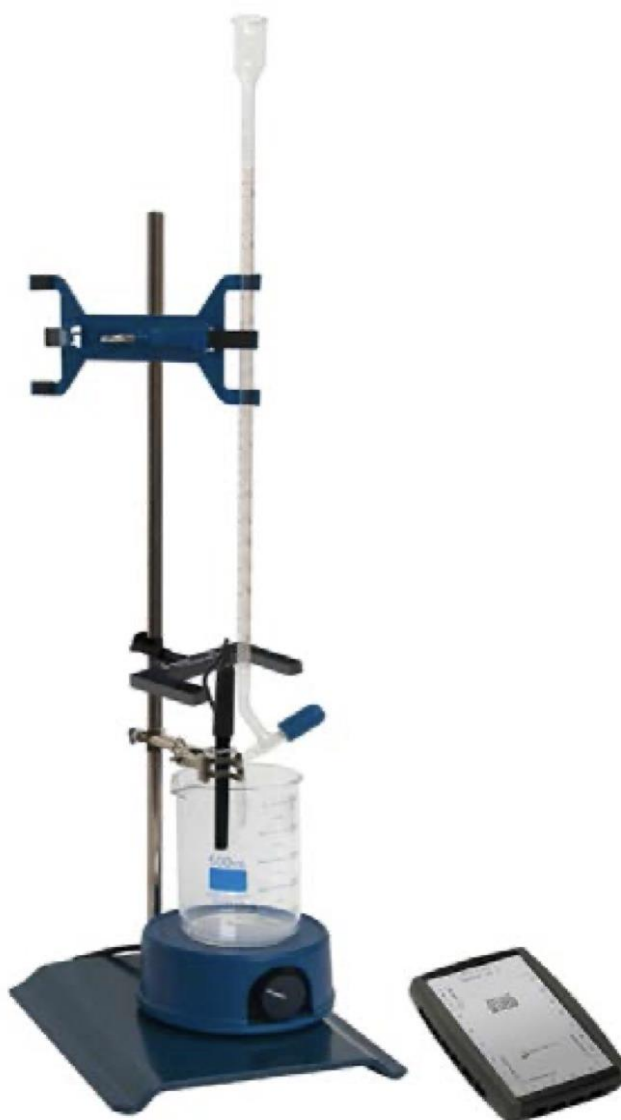
Figure 5.7: Sample analysis by conductometric titration
